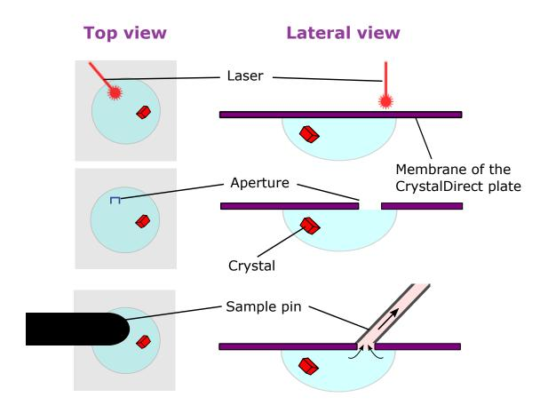
This operation improves the laser cutting quality and according to Pellegrini *et al.*, 2012, risks of mechanical stress to the crystal(s) during the cryo-cooling process are strongly reduced. In addition, diffuse X-ray scattering from vitrified mother liquor is minimized.
