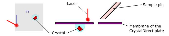
Then, CrystalDirect® cuts the membrane around selected crystals according to the chosen cutting shape.
