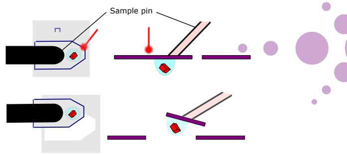
After the laser cutting, the sample is harvested.
