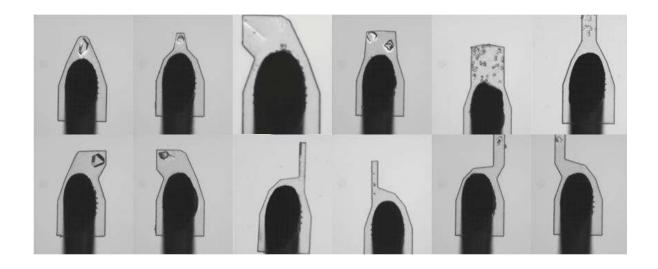
Example of cut shapes available with CrystalDirect ® to harvest single crystals or batches of crystals.
